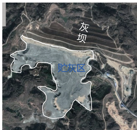
图 8 元家山灰场规划坝高 110 m Fig.8 The planned dam height of Yuanjiashan coal ash storage facility is 110 m
