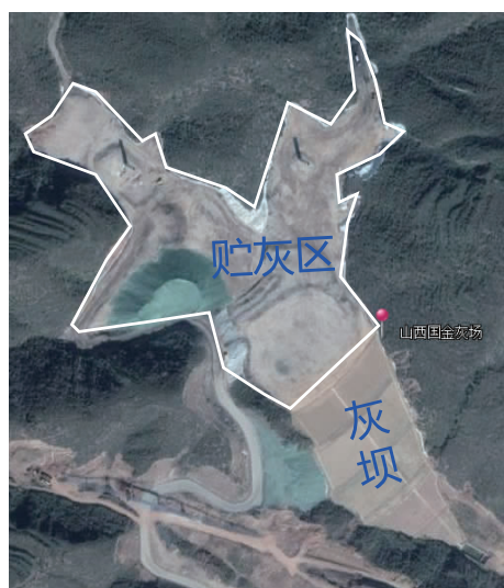
图 9 东沟灰场规划坝高 119 m Fig.9 The planned dam height of Donggou coal ash storage facility is 119 m
